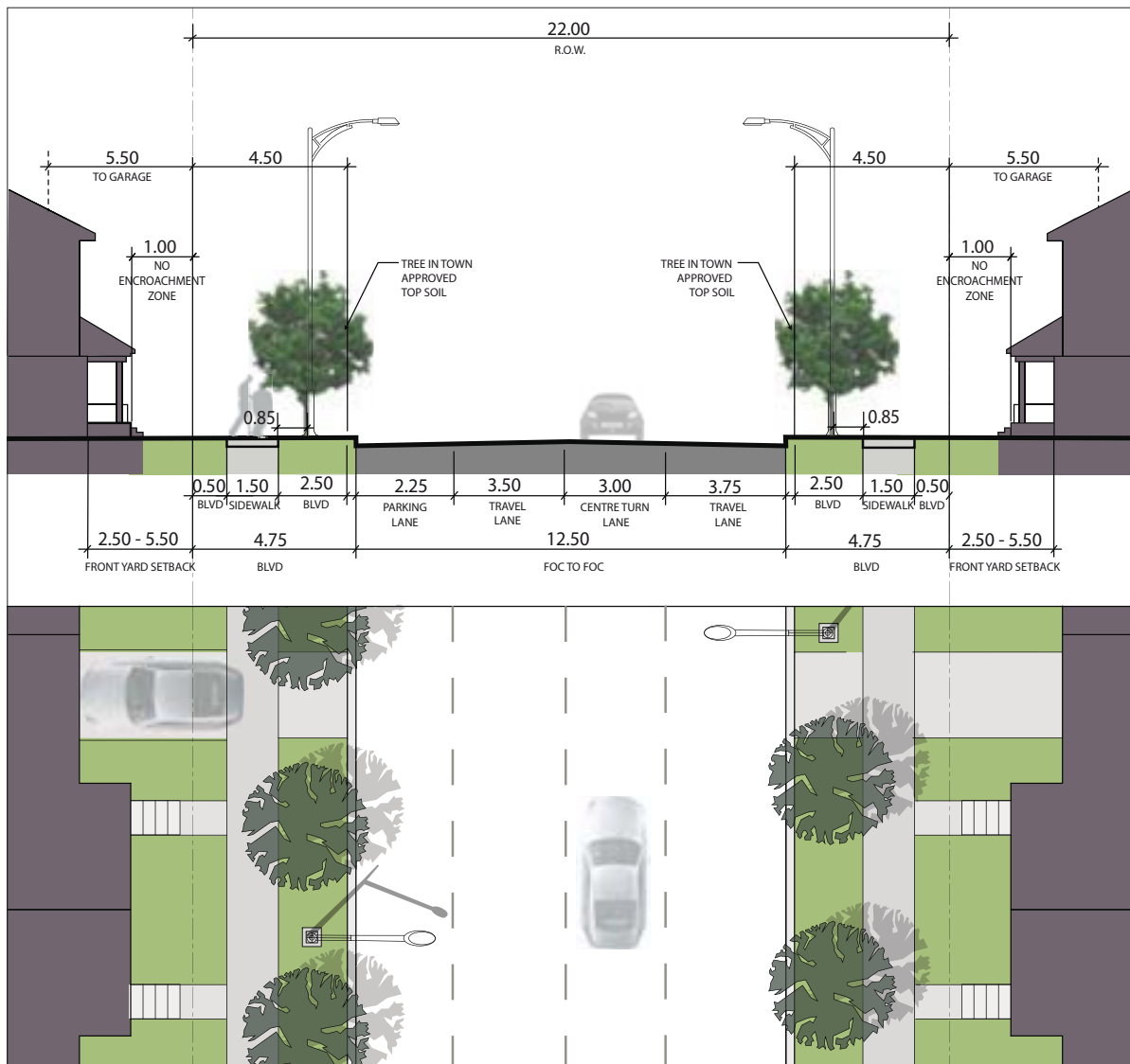
Figure 5.4: Typical Avenue/Transit Corridor section through the General Urban and Sub Urban Design. Street tree height at maturity will vary according to species and the availability of optimum growing conditions (i.e. adequate water, sunlight, soil volume), the protection from compacted soils, salt spray, mechanical damage, pests, and maintenance programs. Please refer to tree habitat design guidelines found in Table 9 of Oakville's Urban Forest: Our Solution to Our Pollution (2006).
