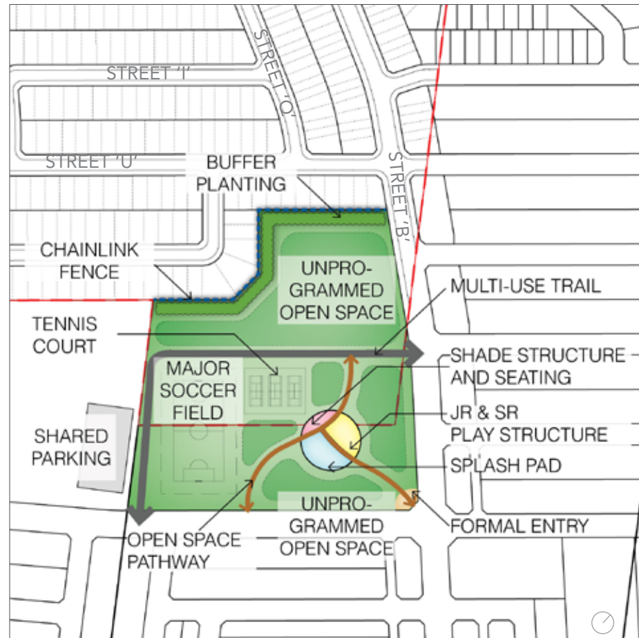
Figure 6.1.1b - Facility Fit Plan for the south Neighbourhood Park with a portion of the park located outside of the Joshua Creek Phase 3 subject lands
