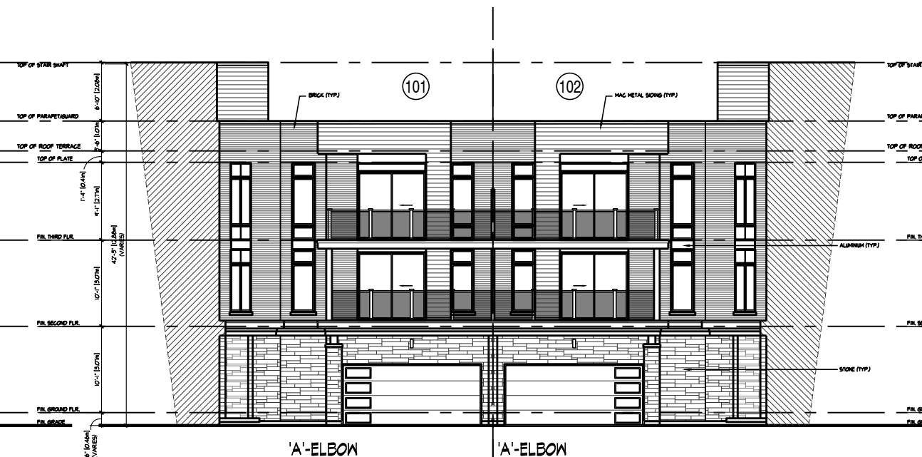
REAR-LANE ELEVATION DUAL-FRONTAGE TOWNS BLOCK 11
