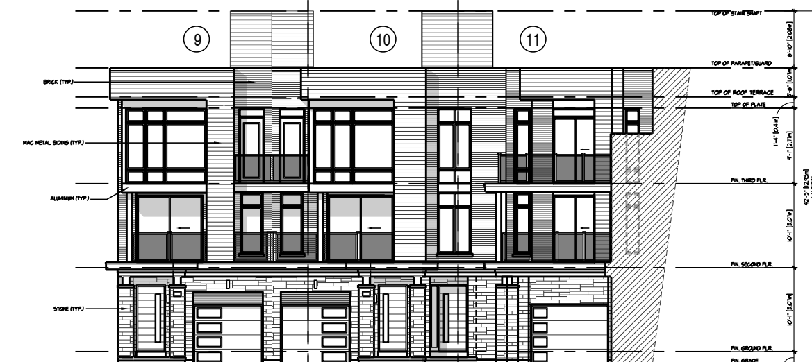
REAR-LANE ELEVATION DUAL-FRONTAGE TOWNS BLOCK 2
