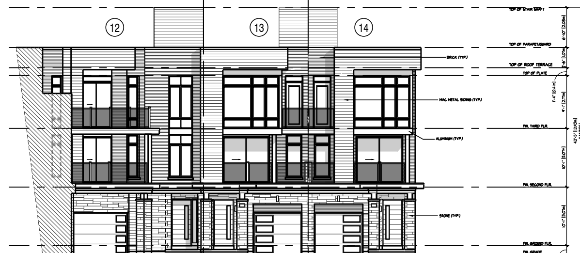
REAR-LANE ELEVATION DUAL-FRONTAGE TOWNS BLOCK 2
