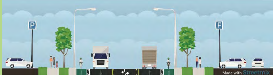
Alternative 3: On-Road Buffered Bike Lanes and Sidewalks
